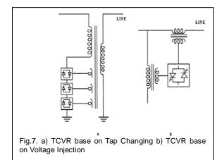
voltage converter for injection of variable ac voltage of the same phase in series with the line in fig. 7b. This is low cost controller can be very effective in controlling the flow of reactive power between two ac systems.
